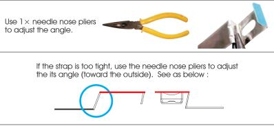
If the strap is too loose, use needle nose pliers to adjust its angle (toward the inside). See as below
